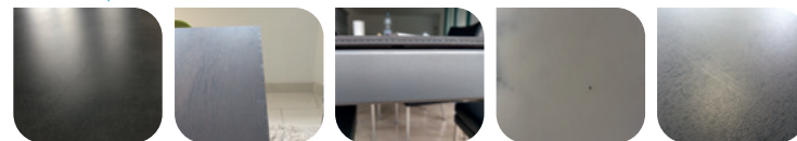
pigmentation spots pigmentation spots irregular glued seams dot stripes
